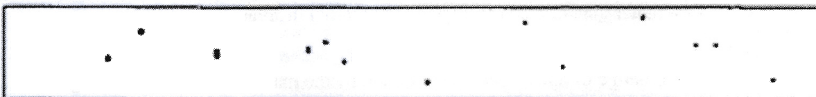
Example 8: Scattered. Three 1/8 in. (0.8 mm), ten 1/64 in. (0.4 mm) discontinuities
